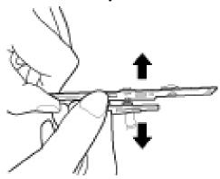
Figure 4-23 Separating fingerprint board assembly
